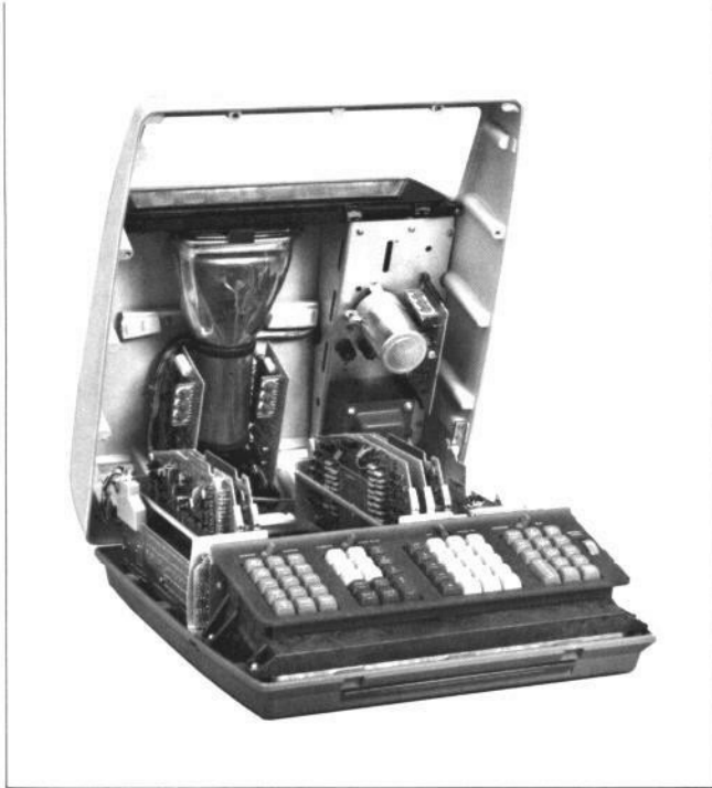
Fig. 5. Internal adjustments of the calculator are easily accessible by removing a few screws and lifting the top.
