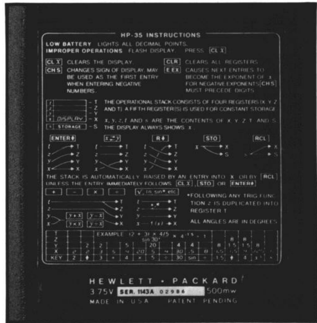
Fig. 2. Instruction panel on back of calculator answers most frequently asked questions.
