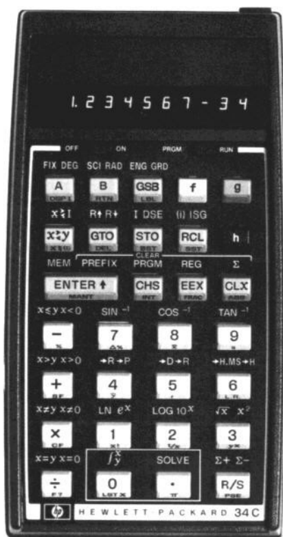
Fig. 2. HP-34C Calculator has keys to solve any equation and to compute integrals.
