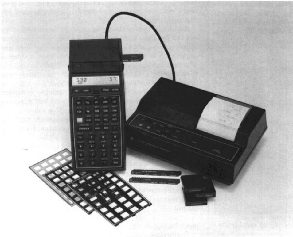
Fig. 1. The new HP-41C Calculator can be expanded like a computer system to include add-on semiconductor memory, mass memory, and hard-copy output. Here the HP-41C is shown with add-on memory modules and its optional magnetic card reader and thermal printer.
