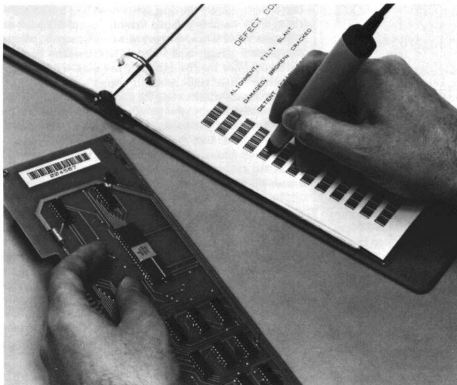
Fig. 1. Illustration of two-out-of-five bar code. Each character is represented by a combination of five bars that are each one or three units wide (see Table I).
