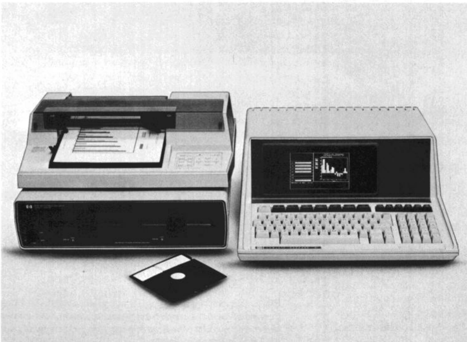
Fig. 3. The HP-87XM Computer is the premier member of the Series 80 family. It features a built-in CRT display and an HP-IB interface for communication with disc drives, printers, and plotters. Its large (128K bytes) internal user memory can be expanded up to 640K bytes by adding RAM modules to its four expansion ports.
