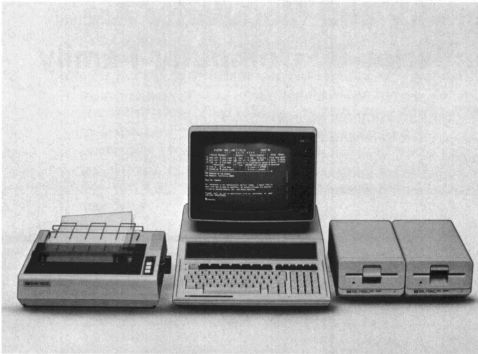
Fig. 2. The HP-86 Computer is the nucleus of a modular computer system. It can drive up to two HP 9130A flexible disc drives and a Centronics-compatible printer directly with its built-in interfaces. Video output is displayed on an external monitor. Both 9-in (82912A) and 12-in (82913A) monitors are available from HP.
