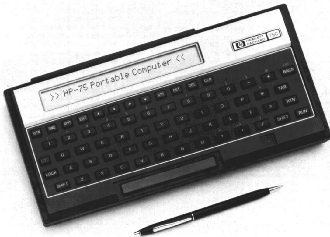
Fig. 1. The HP-75 Portable Computer is battery-powered, has a nonvolatile memory, and provides a wide variety of computational and file handling features in a small package that can be taken with you to solve problems, collect and supply information, compile reports, and even remember appointments.
