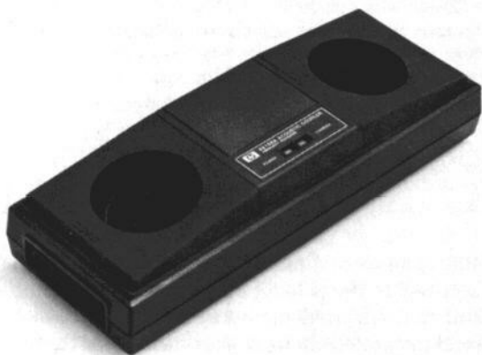
Fig. 1. The HP 82168A Acoustic Coupler can be used to connect any current HP-IL controller such as the HP-75 Portable Computer to a telephone line for transmission of data and programs to another controller or central computer system.
