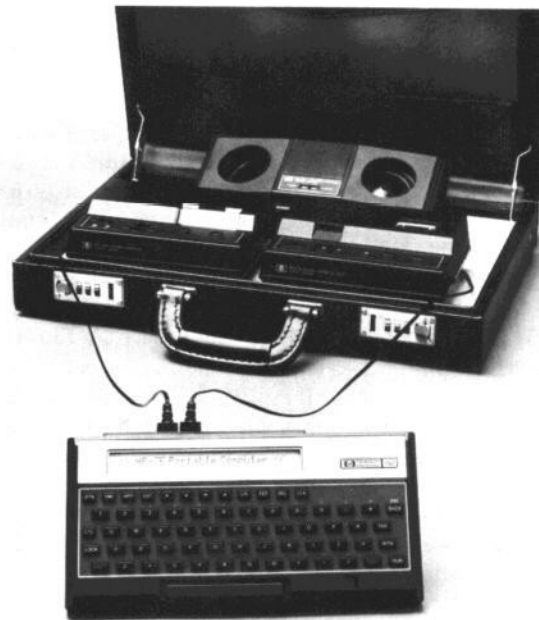
Fig. 2. This HP-75 system features HP's 82168A Acoustic Modem, 82162A Thermal Printer/Plotter, and 82161A Digital Cassette Drive.
