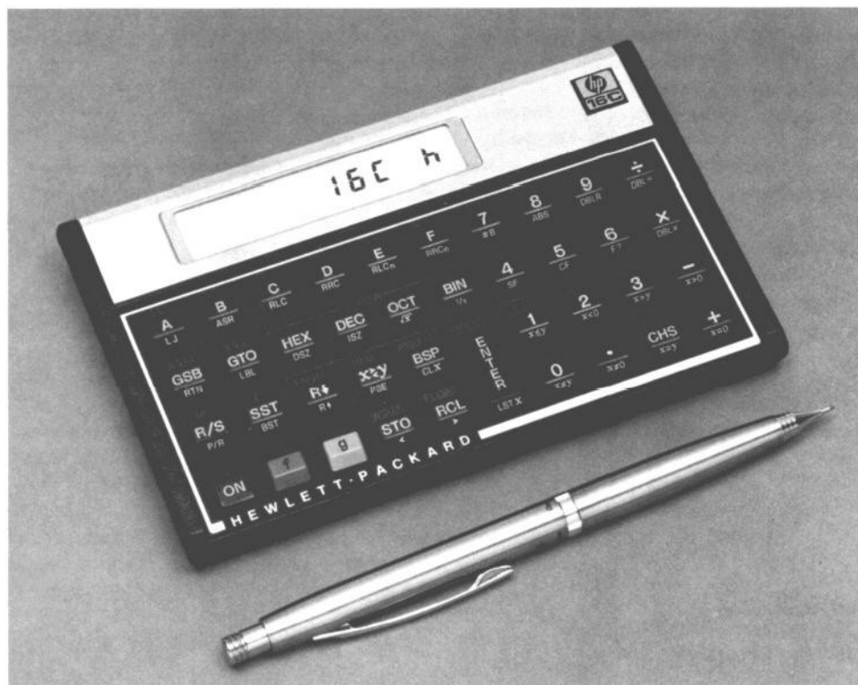
Fig. 1. The HP-16C Programmable Calculator is designed for computer science and digital electronics applications. Besides the normal four-function calculator features, it has a number of capabilities for setting number bases and word sizes, performing Boolean operations, and manipulating bits.
