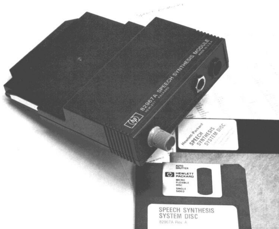
Fig. 1. The HP Model 82967A Speech Synthesis Module provides plug-in speech output capability for HP Series 80 Computers. The speech output can be supplied to headphones, an external audio system, or the speaker contained in the video monitors for HP-86 Computers. Included with the 82967A is a disc containing a 1500-word speech vocabulary and binary routines to simplify the application of speech output to programs.
