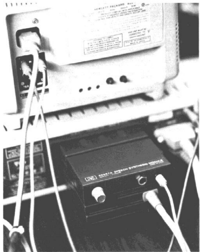
Fig. 4. Installing the 82967A in a Series 80 Computer is a simple process. The module is plugged into one of the four I/O slots in the backplane of the computer as shown and derives its power from the mainframe.
