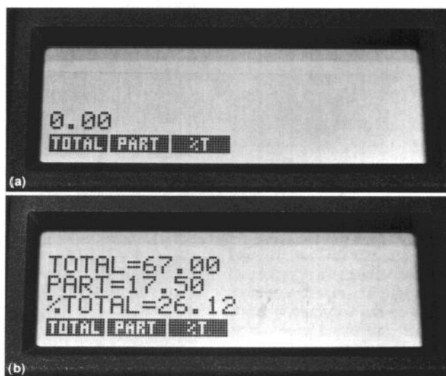
Fig. 4. Use of the HP-18C's softkey user interface. (a) %TOTL menu of BUS application. (b) Answer to determining what percentage of 67 a value of 17.5 is.
