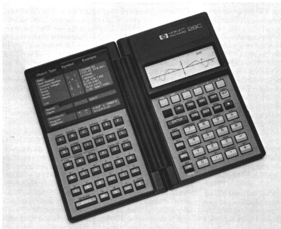
Fig. 1. The HP 28C Scientific Professional Calculator features symbolic entry of algebraic expressions for an extensive range of functions capable of handling real and complex numbers, vectors and matrices, base 2, 8, 10, and 16 integers, lists, and built-in conversion factors. The display can display up to four lines of the indefinite-depth stack or be used to plot functions with a resolution of 32 × 137 pixels. An integral infrared transmitter allows output of data and graphs to an optional printer.
